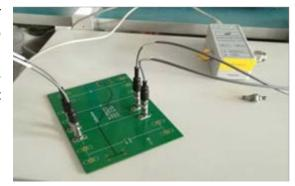
By using the automatic fixture removal function, the measured parts are taken as a whole to extract the balance parameters and to implement 4-port embedded. The test results show that the transmission parameters can be removed well including the near-end and far-end crosstalk.
