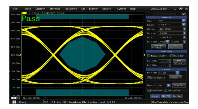
The advanced time-domain analysis option can impose jitter, noise and other interference on the simulation eye map, and simulate the simulation eye map of different positions of high-speed link in the real environment through the addition of correction algorithms such as pre-weighting and equalization.
